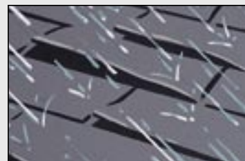
Wind-blown rain trapped under your roof's top layer seeks out those channels.
